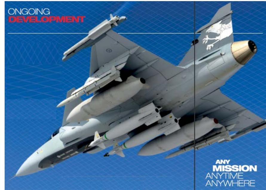
Designed to ensure **outstanding combat agility**. Gripen features a delta-canard configuration with relaxed aerodynamic stability. The delta wing and canards, along with the digital Fly-By-Wire Flight Control System, give the fighter an **optimum combination of maneuverability, acceleration, top speed and short-field performance**.
